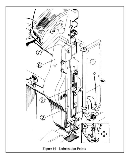
Use a S.A.E. Number 10 oil for lubricating the Number 7 Stitcher. Machines that are in constant operation should be lubricated daily. Machines that are operated periodically should be lubricated just prior to running a job.
