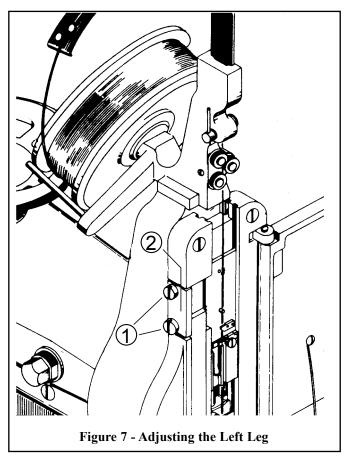
After positioning the Adjustment Rack, tighten the Adjustment Rack Screws (1) and turn the machine over a few revolutions to check the stitches. If the staple is still off center, repeat the preceding steps until a perfect stitch is obtained. With a little experience, the operator will soon learn how much to raise or lower the Adjustment Rack to obtain the correct staple leg length. After the final adjustment has been made, securely tighten the Adjustment Rack Screws (1).
