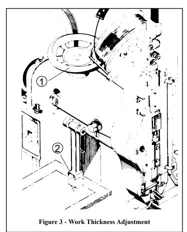
then turn the handwheel to the left, raising the Gauge just far enough to permit work to be withdrawn from between the Gauge and the Gauge shelf. After withdrawing the sample work, turn the handwheel to the right until the Gauge has returned to the point at which it clamped the work.
