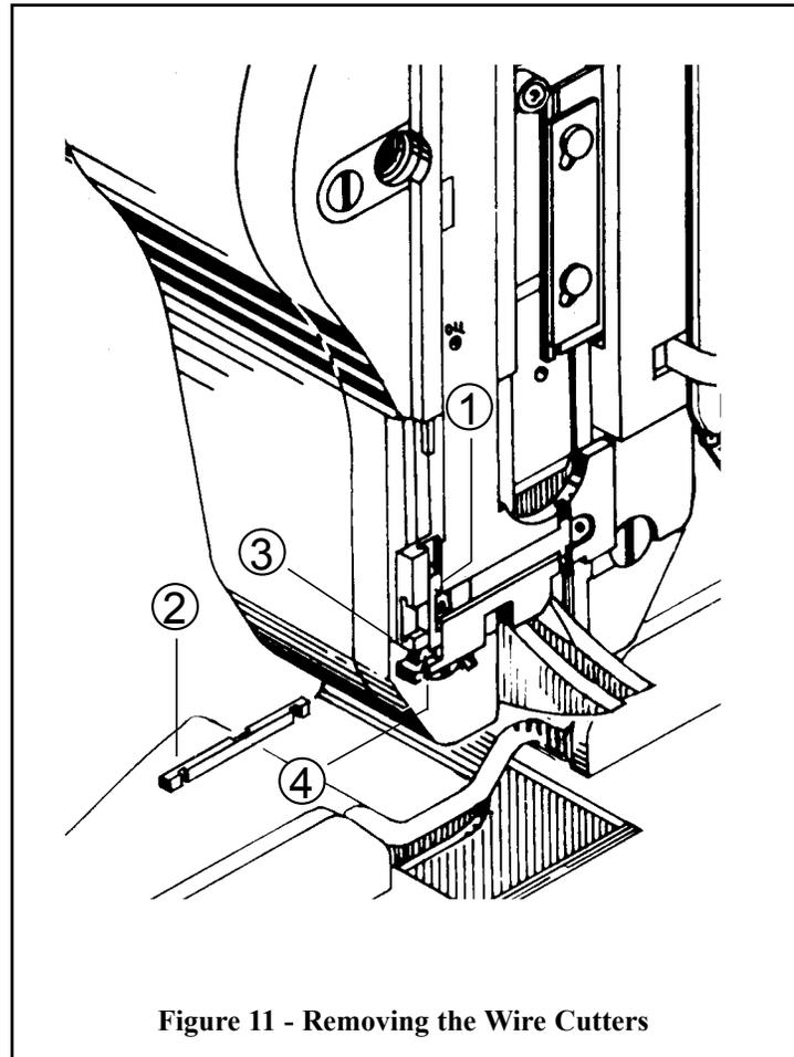
Figure 11 - Removing the Wire Cutters
