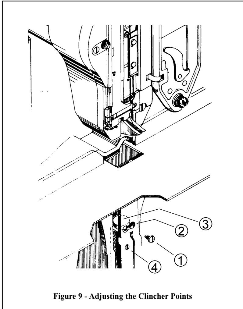
Figure 9 - Adjusting the Clincher Points
