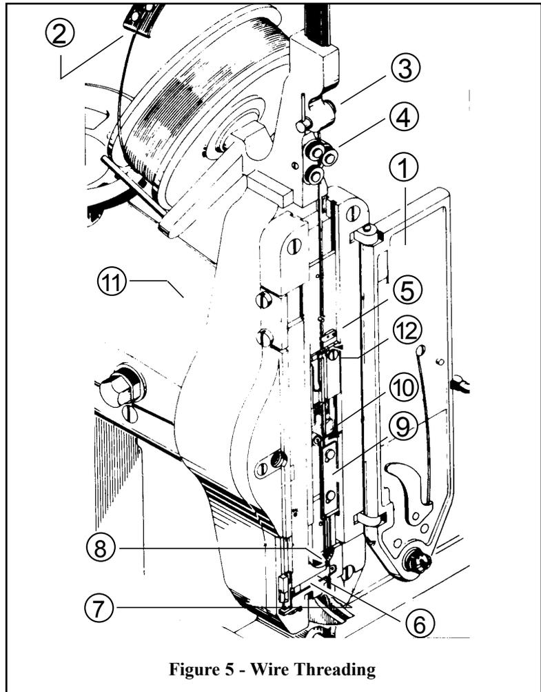
The wire is now threaded in the Head. However, before operating the Stitcher under power, turn the machine over manually a few revolutions and observe that the wire is feeding freely and is being cut off by the Cutters in the Cutter Holder. Then close the stitcher head door and check that the wire is feeding in a straight vertical line, as directed in the following paragraph.
