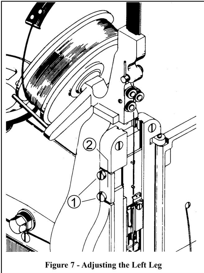
Figure 7 - Adjusting the Left Leg
