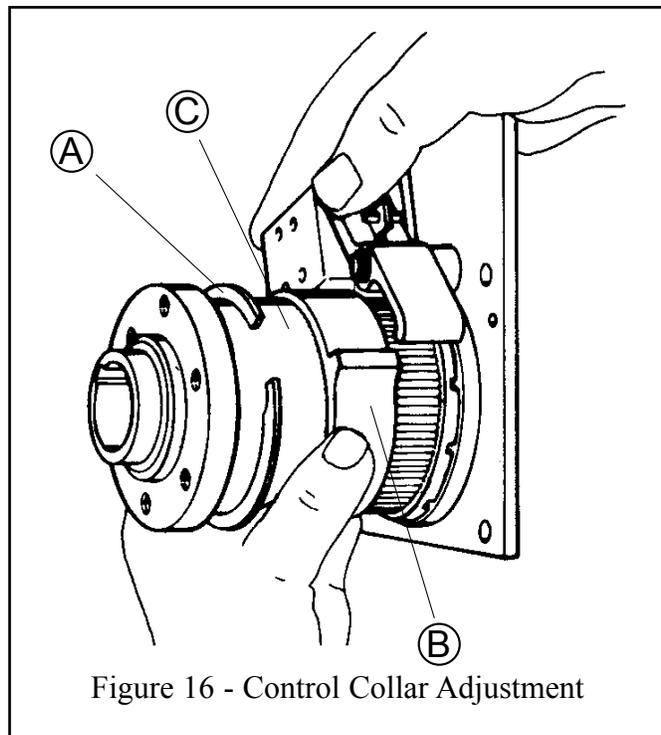
Figure 16 - Control Collar Adjustment
