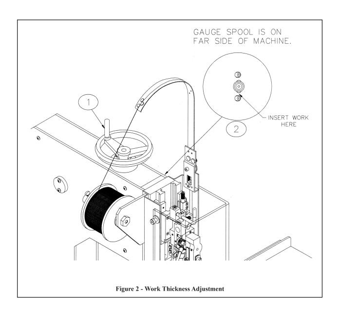
If the Machine is operated on work thicker than is set to handle, damage will result and the Stitcher will not operate properly.
